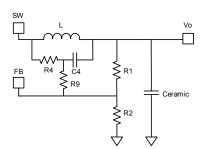
Figure 11: Simplified Circuit of Ceramic Capacitor
