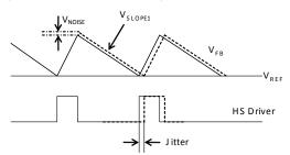
Figure 4: Jitter in PWM Mode
