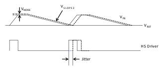
Figure 5: Jitter in Skip Mode
