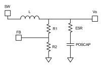
Figure 10: Simplified Circuit of POS Capacitor
