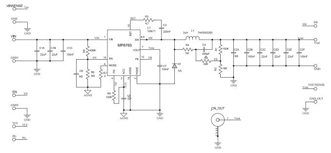
Note: Recommend to pull-up PG to IC VCC pin. If need pull-up PG to external power supply, please refer to the PG description in application information section.
