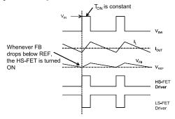
Figure 2: Heavy Load Operation
