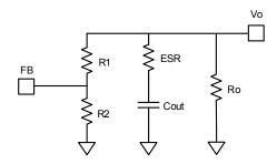
Figure 8: Simplified Circuit in skip Mode
