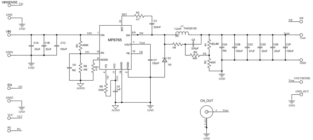
Note: Recommend to pull-up PG to IC VCC pin. If need pull-up PG to external power supply, please refer to the PG description in application information section.
